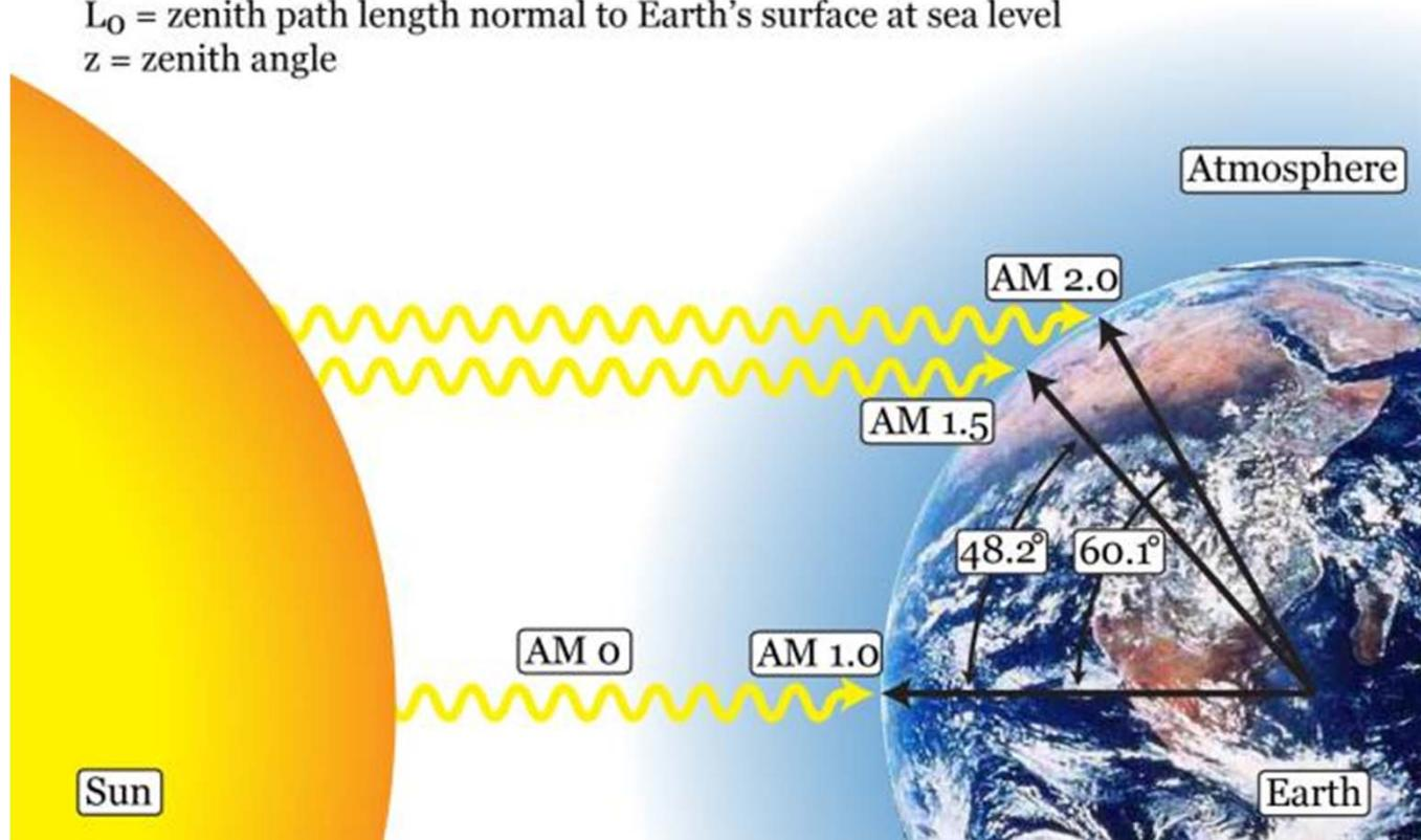
**AIR MASS defines the *power density* and the *spectrum* of incoming radiation**
